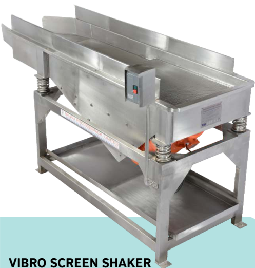
VIBRO SCREEN SHAKER For removal of excess moisture from surface of washed whole/cut fruits and vegetable before further processing. Available from 100-2000 kg/hr capacities
